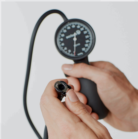
Picture 7: Press the metal plate in so that the small metal split protrudes.
